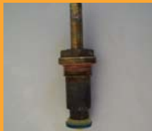
F. The metal tap body. The beige and greeny/blue bit at the bottom is the washer.
